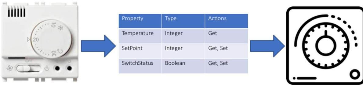
Figure 1 – Mapping a physical object to its digital twin
