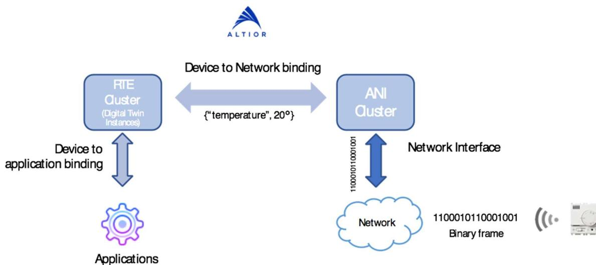
Physical objects (devices and sensors) implementing the open source Altior API for devices also have the capability to define a redundant network interface and service configuration which can be switched automatically in the case of a primary network failure.
